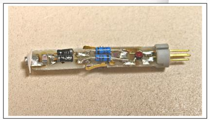
A small clip lead should be used to clamp to the gold fingers at the middle of the board and ground those to the metal shell to the right of the board. Be careful not to damage these since they ground parts of the circuit when it is inserted back into the metal housing. Note on the drawing above that I have labeled the FET source on pin 1 and the drain on pin 4. The schematic shows that the source should be -2.3 V and the drain at -17 V. Measure these voltages with a DVM with no signal applied.
